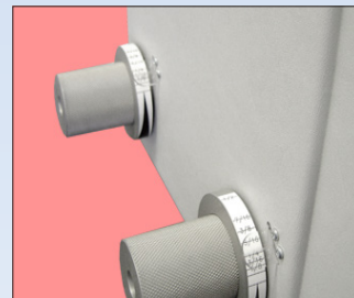
Nip & Pull Roller Adjustment
