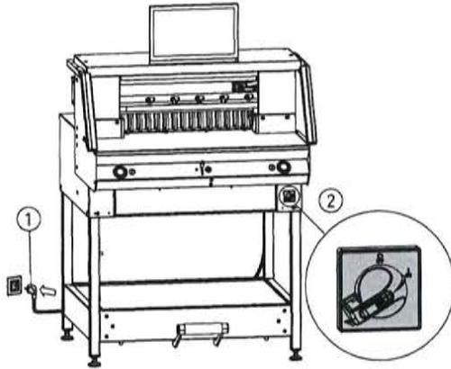
Plug in power cable ① at the power socket.
