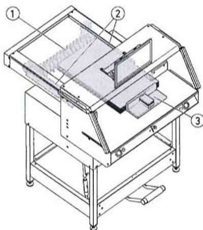
Paper installation at the back gauge (1) and side stop to the left and right (2). Use the provided paper knock-up block (3) for adjusting paper stacks. (Move back gauge forwards before turning the stack of paper).
