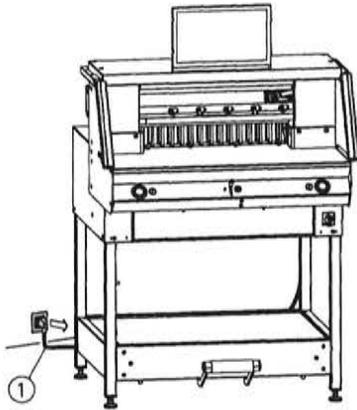
Protect the power cable ① from heat, oil and sharp edges!
