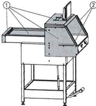
Dangerous machine parts are protected by guards and covered by panels ①. The machine may only be operated with all safety and panelling sections fitted and in particular with:
