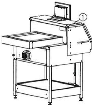
For specific technical data, please refer to the information on the identification plate ① of the machine. To file a warranty claim, the device must still bear its original identification plate.
