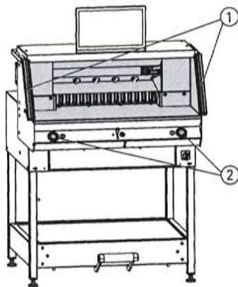
The dangerous cutting movement is protected by a safety light beam curtain ① and a two-hand cutting ② activation!
