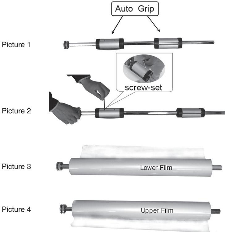
1. As shown in picture 1, insert auto grips onto the upper/lower film shaft.
