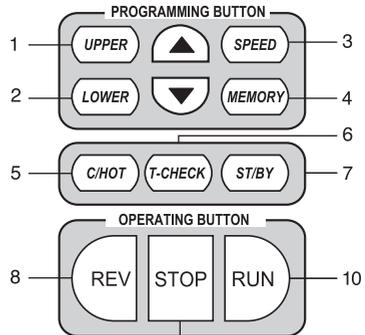
5. **C/HOT:** To change the mode from hot to cold or cold to hot lamination. In cold mode, the speed defaults to 2 (speed 1~4 settings) and stand-by function is disabled.
