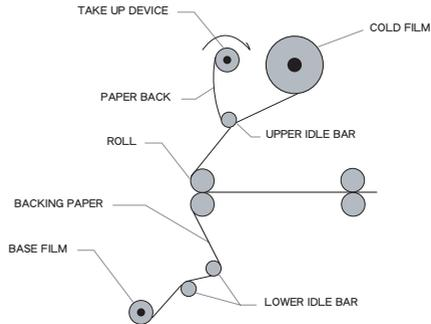
1. Follow the steps in the "Loading Film" procedure by loading the upper shaft with pressure sensitive film, e.g. (Royal Print-Pro Film) and lower shaft with pressure sensitive mounting adhesive films or backing paper (Royal Sovereign White-Mount or Clear-Mount).
