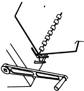
**2** Measure the thickness of papers to be bound and determine punching depth by using binding gauge. Select correct diameter of binding comb to use.
