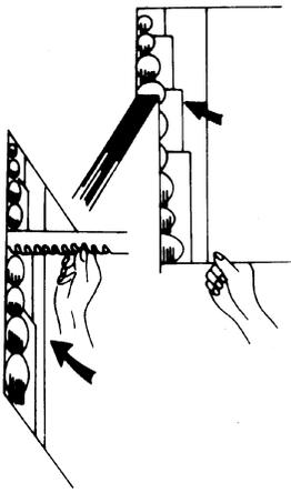
**4** Insert paper into punch throat. pull handle down to punch. Return handle to upright and pull paper out. Continue this step until all papers are punched.
