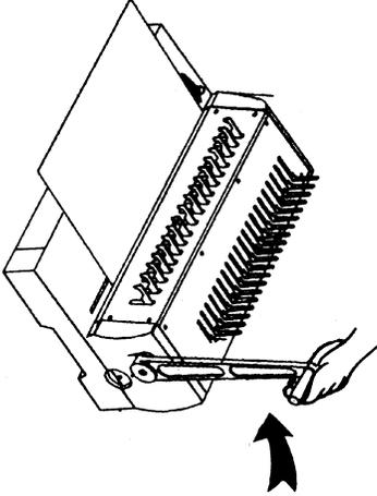
**6** 1. The binder stop is on the left hand side turn it down forward to the extreme end.
