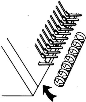
**7** Insert papers vertically and make sure all fingers are line up with punched holes lay down papers horizontally. Continue this step until all papers are bound.
