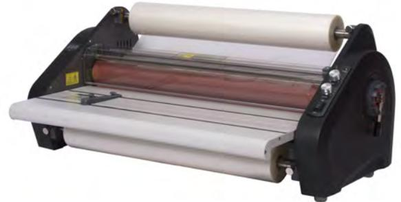
With safety and energy savings concerns in mind, the Phoenix 2700 includes the latest innovations. Safety measures include safety latches on the feed tray and a safety shield preventing the unit from running if they are not in place. To conserve energy, the machine will drop into a standby mode (176°) if unit has been idle for 3 hours. If there is no activity on the unit for 4 hours, the heaters turn off.
