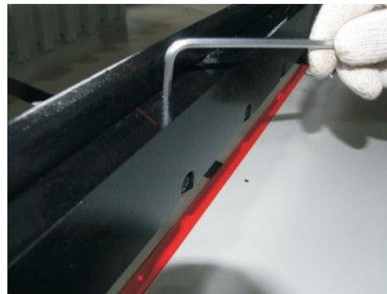
2. Loosen the seven M6 fasten screws and adjust the screws on the blade carrier until the blade cuts into the cutting stick by about 0.3 – 0.5mm.
