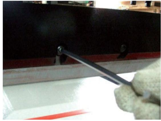
1. Use a Phillips head screwdriver to remove the screws that hold the upper cover in order to access the cutting blade.
