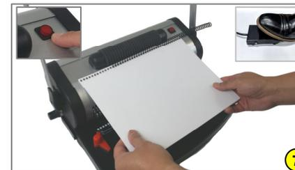
7. Press the coil inserting roller switch to the ON position or use the foot pedal to spin the roller, then grasp the document and gently press against the coil against the roller. TIP: You may prolong the life of the roller by using the foot pedal more frequently.
