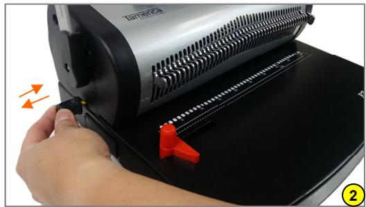
2. Adjust depth margin control from 2.5mm to 6.5mm. This controls how far or how close you want the holes to be in relation to the edge of the document.
