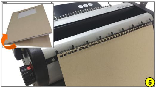
5. Position the wire on the wire holder. TIP: Flip the back cover over to make it face the front (see inset) then insert into the wire making sure all teeth go through the holes.
